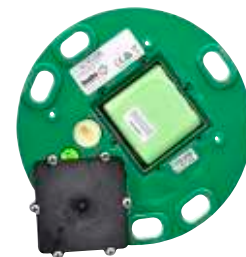
Internal user-replaceable battery in sealed battery compartment
